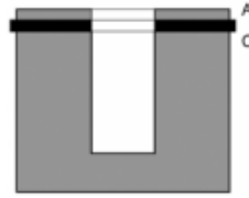
Figure 7: Schematic of a typical microhollow cathode discharge (MHCD), with a cylindrical cavity in the cathode, from [28].
